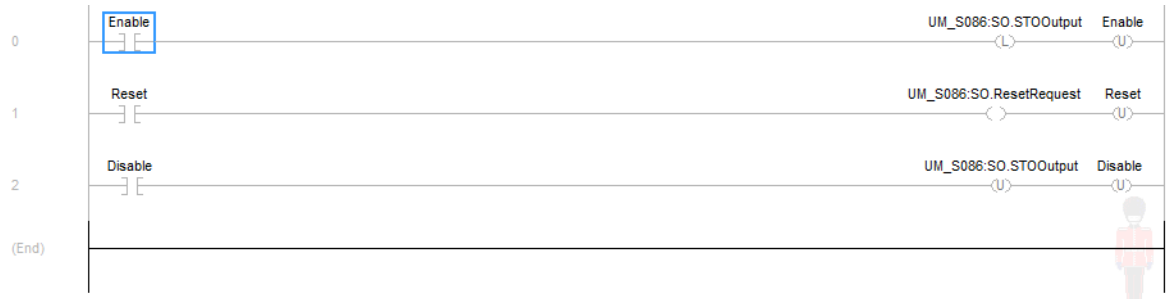
Figure 148 - STO Function with Safe Stop Only-No Feedback (Logix Designer, version 31 or later)
